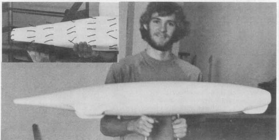
(Fig. 4) No. 1A showing how the bottom rear has been brought down to eliminate the wheel pants and large separation area. The yarn tufts are for flow visualization in the wind tunnel.
