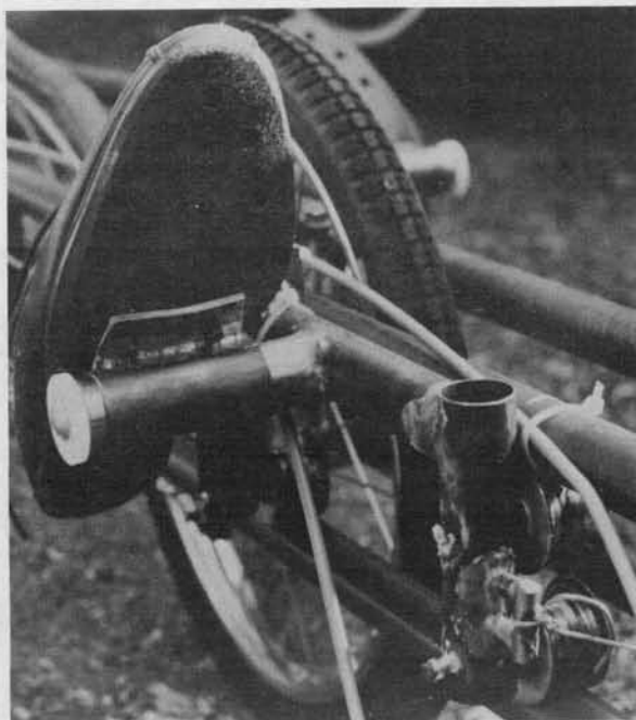
Close-up of pedal. Note aluminum rollers and pull-back cable.
