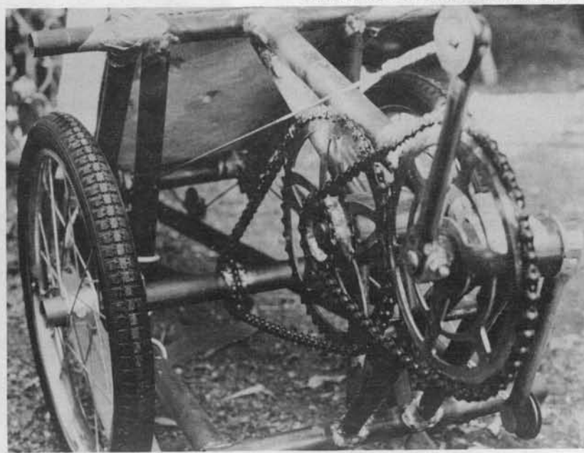
Final drive. Chains in series provide 90 rpm at 50 mph. No freewheel, no brakes!
