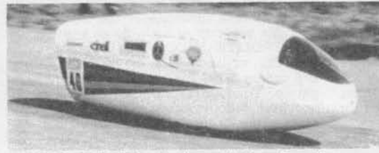
Ken Bird's GENESIS, with "Kamm" tail configuration.
