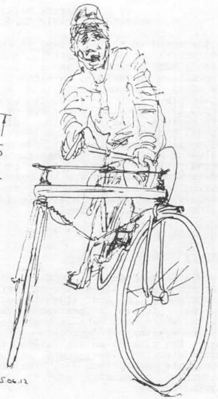
Tricycle 3, with articulated frame, greatly reduced lower-back stress.
