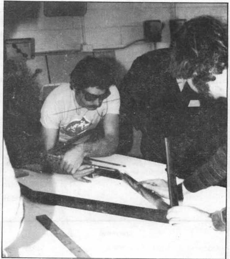
Welding instructor Stephen Delaire tack-brazes the "class project" frame together. Frame is built of oval-section tubing.
