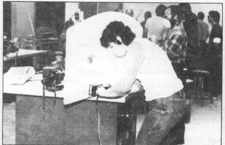
Welding instructor Stephen Delaire tack-brazes the "class project" frame together. Frame is built of oval-section tubing.
