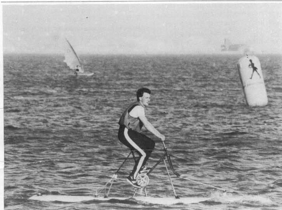
Craft (not "Daring") brought to Johnnie Walker Speed Sailing Week by David Whitt, Oxford University, developed by Johnathan May and David Whitt. Conventional sailboard as hull. Note position of front rudder. Photo courtesy of Johnnie Walker.
