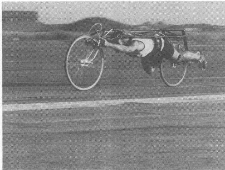
Allan Abbott on his first prone recumbent bicycle which was designed to minimize frontal area.
