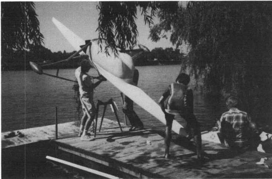
Hydroped III being removed from Lake Adrian. Notice aerodynamic cowling over cockpit. Builder, Sid Shutt is at left.
