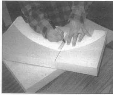
Figure 4. After the posterboard templates are cut out, the chassis cut-out is traced onto the Styrofoam blocks.
