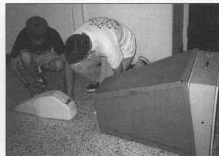
Figure 3. Aaron and John test their creation in the "wind tunnel", a box fan fitted with a cardboard nozzle.
