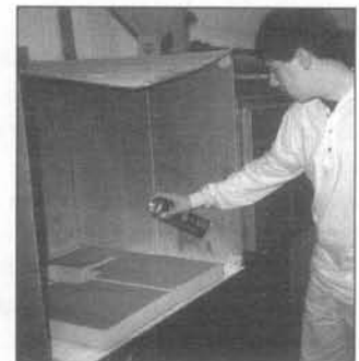
Figure 6. Applying adhesive to the Styrofoam
