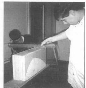
Figure 7. Cutting the foam block on two planes (plan and elevation)
