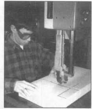
Figure 5. John cuts out the chassis opening in a 50-mm thick Styrofoam piece.
