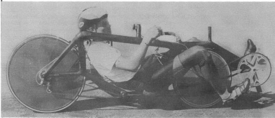
*The first model Cutting Edge shown above has an asymmetric carbon frame with a suspended sling seat, stabilized by cross ties. The second model, as yet uncompleted, has a front-wheel drive.*
