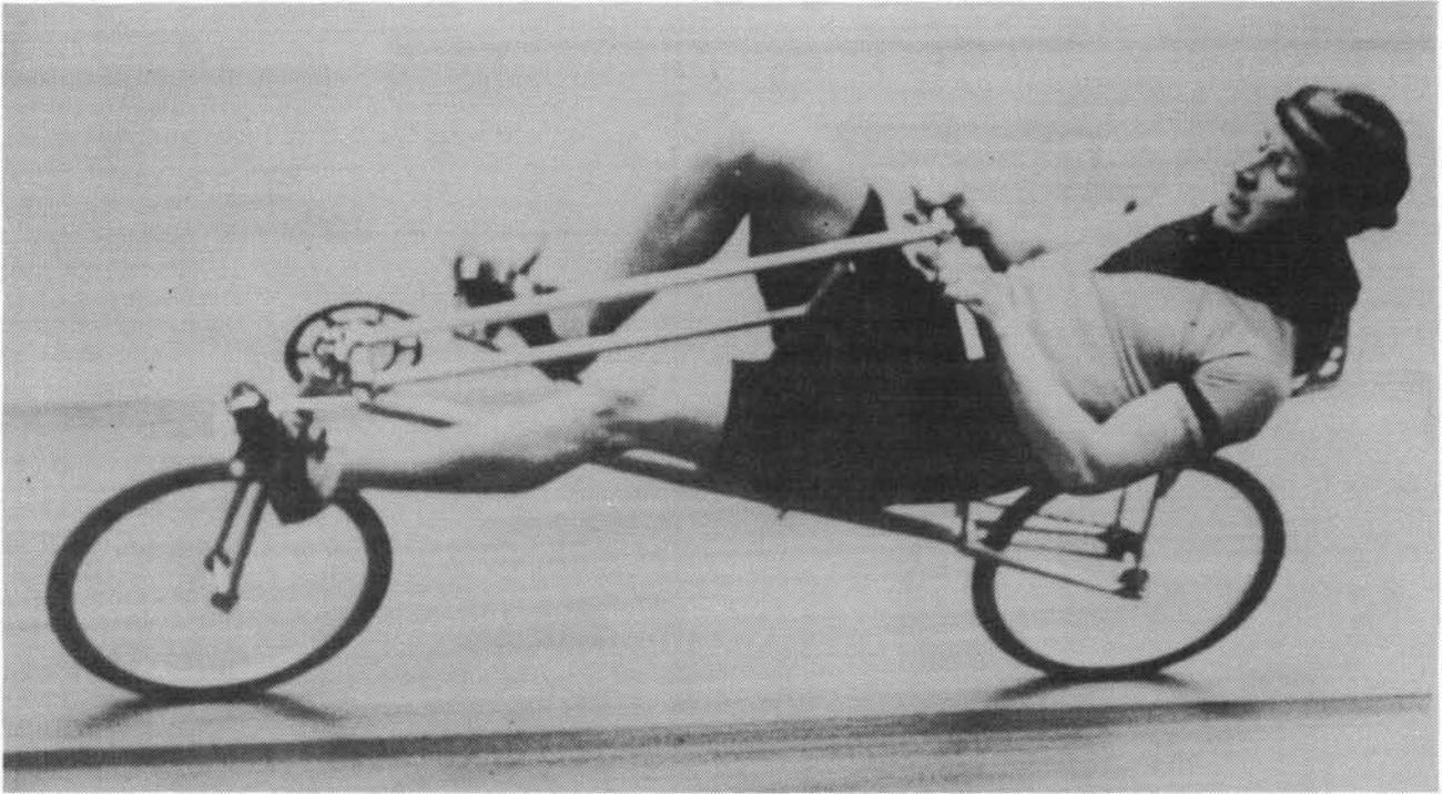
*Francis Faure breaking the world hour record in 1933. See Arnfried Schmitz's fascinating article starting on the next page. (Editor's note: why aren't more recumbents made today with this attractive configuration: mid-length wheelbase with the pedalling axis over the front wheel; rear wheel of equal size; steering through a universal joint; straight chain line to back wheel and simple linear frame?)*
