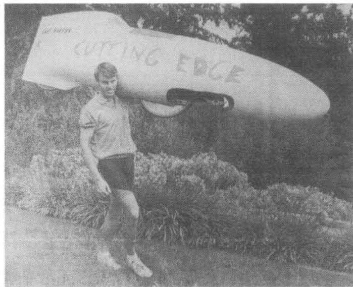
*Matt Weaver and the Cutting Edge. The front wheel is well back so that sidewind pressure will cause the bike to lean into the wind for stability. The fairing was designed for a linear drive; however, a circular crank made it necessary to cut openings for the knees and heels. Stretched, latex sheet normally covers the openings. In this photo, the bottom openings are not covered.*
