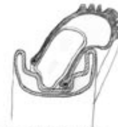
Figure 4. Tire with beads having slipped off the bead set flops over first on one side, and then on the other.
