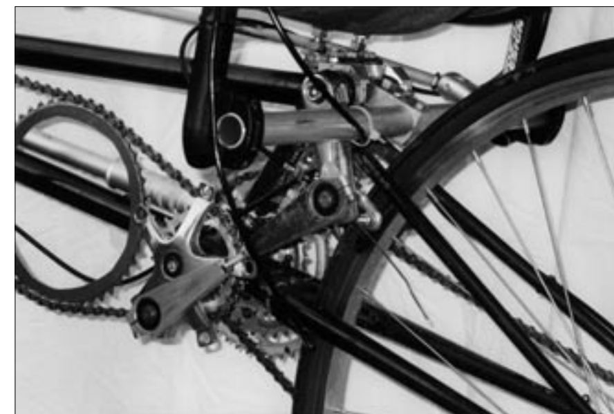
Figure 2. Close-up of the arm powered rowing/steering mechanism
