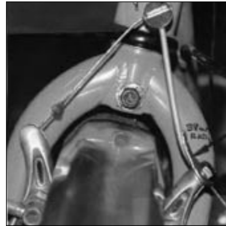
Figure 3. Cantilever brake with curved washer installed, showing gentle curve through which the cable is now bent.
