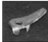
Figure 2. Curved washer (above) made to fit under the clamp bolt on the cantilever arm, providing a large-radius bend for the cable.
