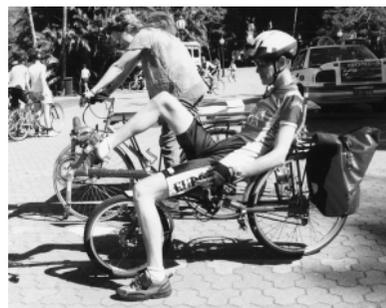
semi-recumbent designs. The real question you are asking is, will you be faster on a recumbent? The answer is, "maybe". There are so many factors involved; how long you've been riding, how long you've trained on the recumbent, style and weight of the bike, topography - hilly, mountainous, flat. Since the biggest factor limiting speed is aerodynamic drag, if you want to go really fast, use a recumbent with a well-designed fairing or a full body. In this case, the answer is YES, they are
