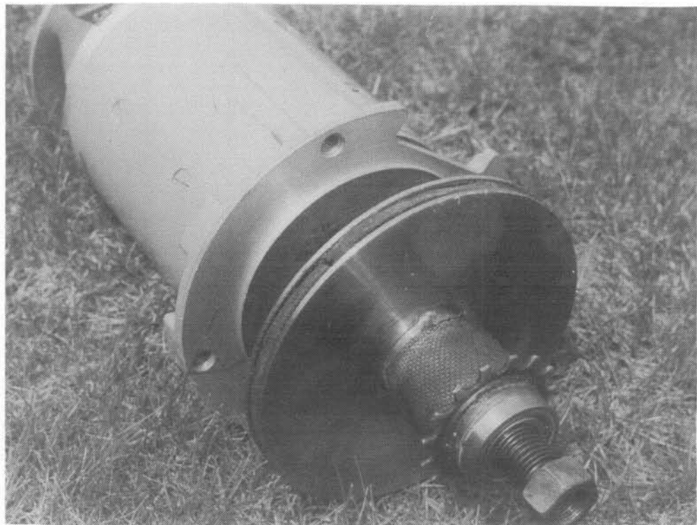
▼ FIG. 4 DC Drive motor and constant-torque slipping clutch. PHOTO BY: Dave Wilson
