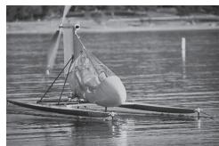
he pedal and propeller powered hydrofoil Decavitator sliced through the water at 18.50 knots (21.28 mph)
